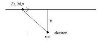
First consider an interaction of a particle of charge Ze with an electron, as shown. We take t = 0 at the time of closest approach. To first order, the path of the particle remains straight, and the horizontal component of its electric field does not have any net effect on the electron. The perpendicular electric field component produced by the moving particle at the position of the electron is (notes 2 pg 6):
